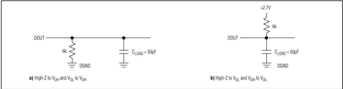
Figure 1. Load Circuits for DOUT Enable Time
