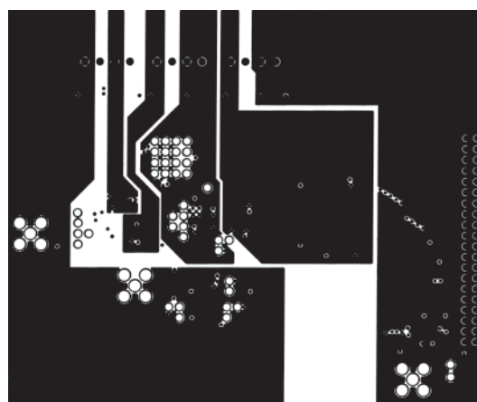
Figure 15. PCB Ground Layer—Layer TBD
