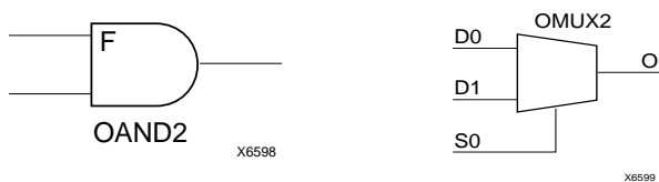
Figure 20: AND & MUX Symbols in XC4000X IOB
