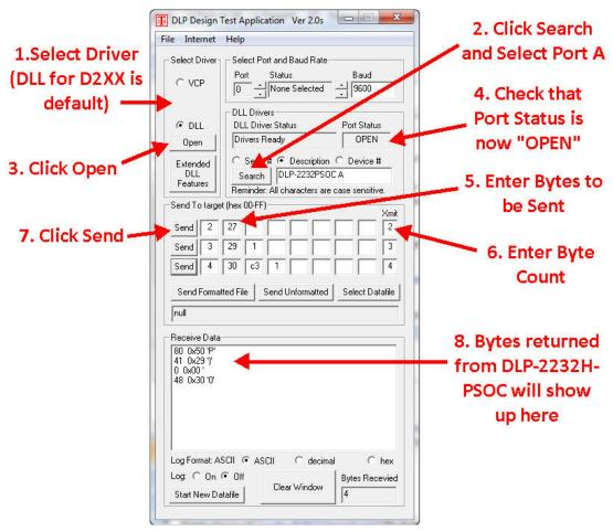
The commands used to interface to the DLP-2232H-PSOC5 are detailed in Section 10 of this datasheet.
