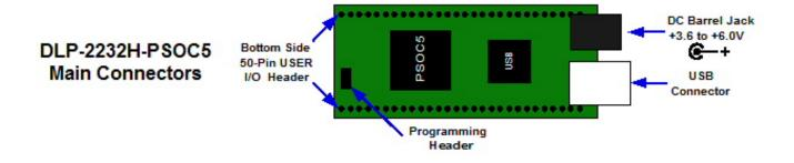
Connection to user electronics is made via a 50-pin, 0.9-inch wide, industry-standard 0.025-square inch post DIP header on the bottom of the board. The bottom side 50-pin header provides access to the user input/output pins as well as the USB port power output and the module's power input. The bottom side header mates with a user-supplied, standard, 50-pin, 0.9-inch spaced DIP socket.
